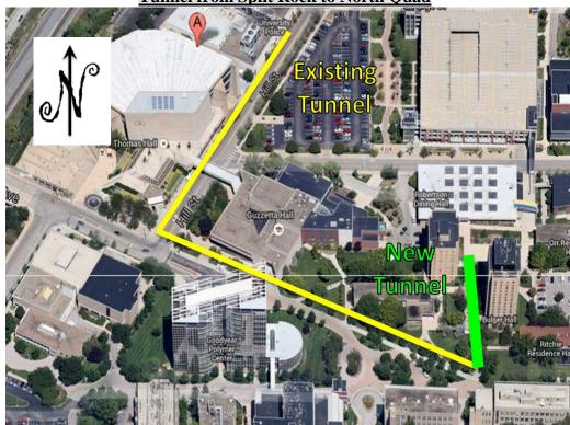
New Proposed Tunnel Construction Site Plan- new Tunnel from Split Rock to North Quad with construction limits
